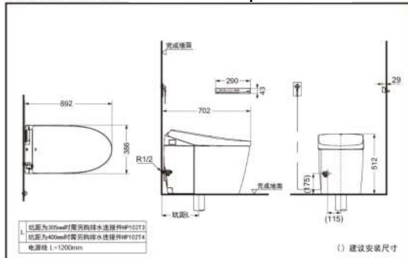
**CES8E810GCN****Function part****TCF8E810GCN#W****Toilet part****CS921B-8E810#XW****Toilet drain****HP102T3#00****HP102T4#00****FEATURES**
